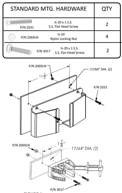
FIGURE 1 (Thru Mounting Method)
