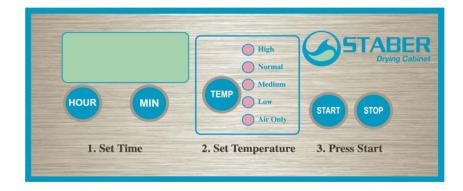
**Temperature Settings**: A simple touch of the TEMP pad on the control panel allows a total of five preset drying temperature settings, with associated LED light indicators. The five different drying temperatures are: **Air Only** (No Heat), Low (105F), Medium (120F), Normal (135F) & High (150F).
