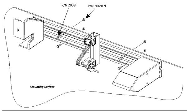
STEP 2 — Attach bracket to mounting surface (PAC TRAC)
