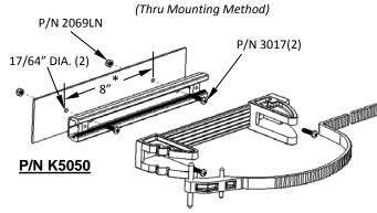
Additional holes may be required to suit application and avoid interference with channel nuts.
